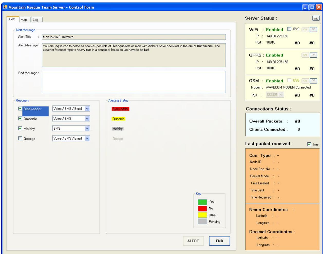
**Figure 4 The Alert tab page of the Control Form of the server application**
