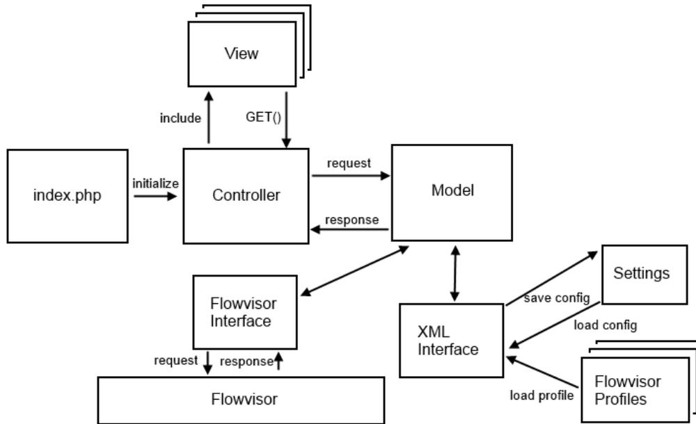
Fig. 3. HomeVisor Components and Interaction
