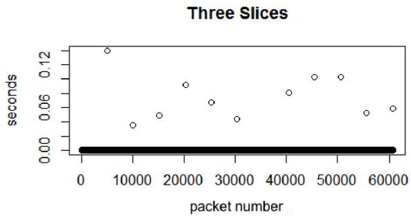
Fig. 6. Inter-packet delay measurements in three slice setup
