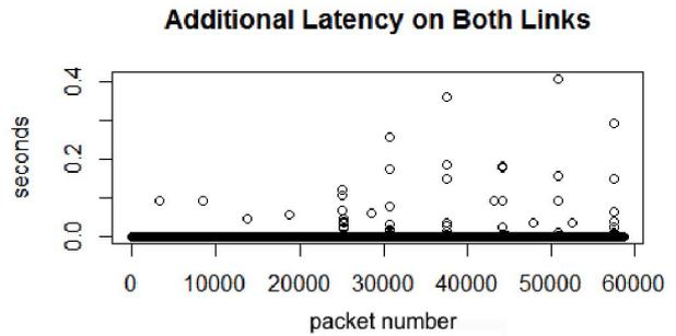
Fig. 8. Traffic behaviour when high latency is introduced between the data and control plane. 100ms is introduced between the switch and the FlowVisor and 100ms is introduced between the FlowVisor and the controller.
