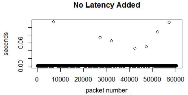
Fig. 7. Traffic behaviour when no additional latency is introduced between the data plane and the control plane.
